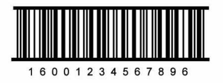
It should be noted that the width of each bearer bar need be only twice the width of a narrow element. The bearer bars in this instance are not required to completely surround the symbol, only at the top and bottom of the symbol. The bearer bars do not need to extend into the clear margin.
