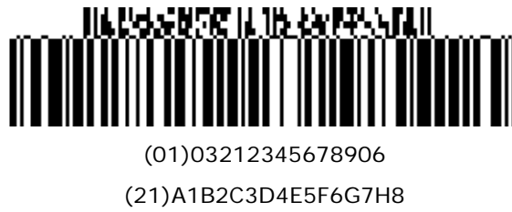
Figure 5.11.8-9. GS1-128 symbol with a four-column CC-A
