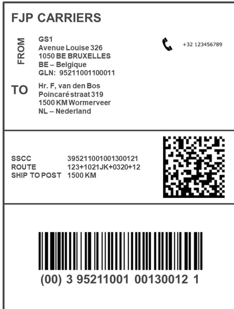
Figure 6.6.5-8 Label GS1 DataMatrix encoding transport process information
