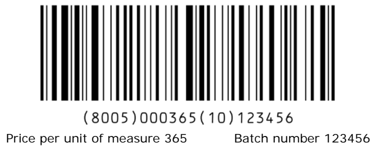
Figure 7.8.6.2-2. Data encoded in one concatenated GS1-128 symbol
