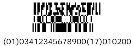
Figure 5.11.8-6. GS1 DataBar Stacked symbol with a two-column CC-A
