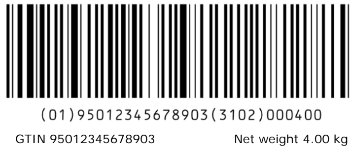
Figure 7.8.6.1-2. Data encoded in one concatenated GS1-128 symbol
