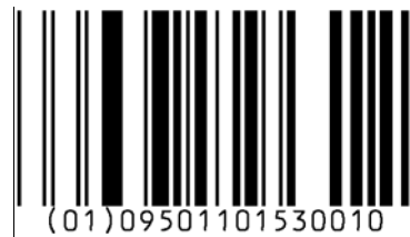
Figure 5.5.2.1.1-1. GS1 DataBar Omnidirectional barcode
