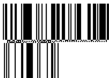
Figure 5.5.2.3.2-1. GS1 DataBar Expanded Stacked barcode
