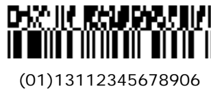
Figure 4.15-2. HRI with some of the data omitted
