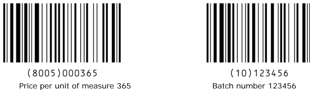
Figure 7.8.6.2-1. Data encoded in two GS1-128 symbols
