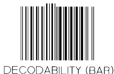
Figure 5.12.5.12-3. Calibration symbol with engineered low decodability grade
