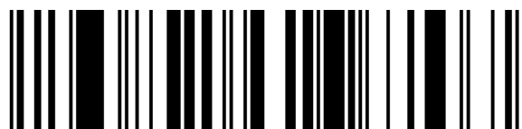
Figure 5.5.2.3.1-1. GS1 DataBar Expanded barcode
