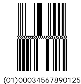
Figure 5.5.2.1.4-1. GS1 DataBar Stacked Omnidirectional barcode
