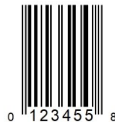
Figure 5.2.2.4-1. UPC-E barcode (encoding 012345000058 by zero-suppression)
