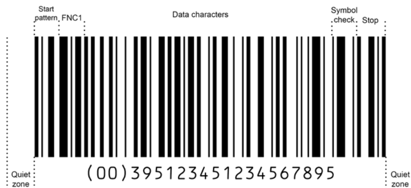
Figure 5.4.2-1. General format of a GS1-128 barcode
