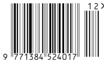
Figure 5.2.2.5.1-2. EAN-13 barcode with two-digit add-on symbol
