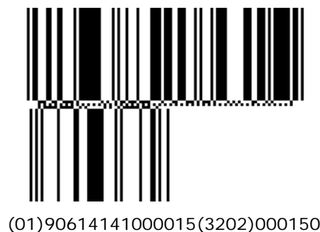
Figure 7.8.6.3-1. Example of GS1 DataBar Expanded Stacked barcode that uses concatenation
