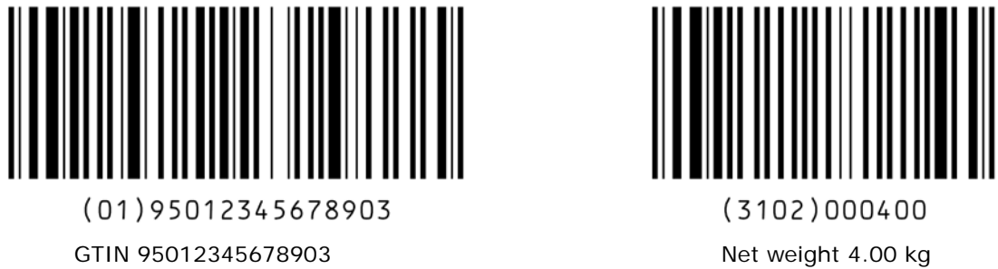
Figure 7.8.6.1-2. Data encoded in one concatenated GS1-128 symbol
