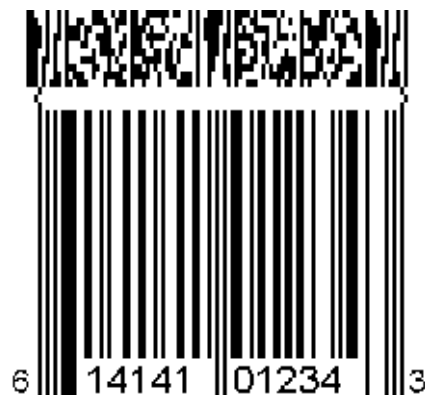
Figure 5.11.8-2. UPC-A symbol with a four-column CC-B component
