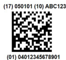
Figure 5.1-6. GS1 DataMatrix barcode
